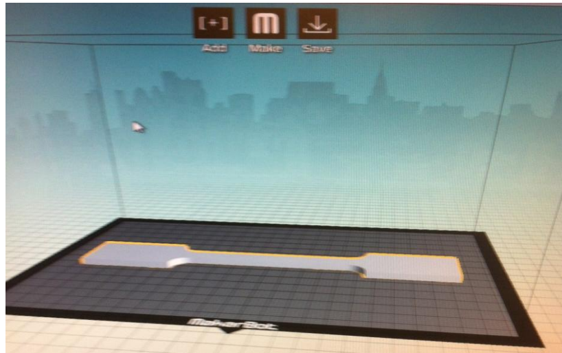
Figure 2. Test sample imported using Maker ware software
