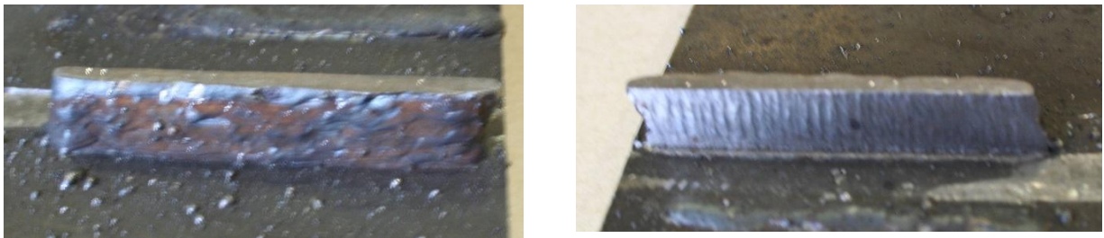
Figure 4. 3D printed wall before (left) and after (right) machining
