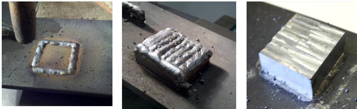
Figure 5. 3D metal printing and machining of hollow box
