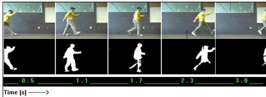
Figure 5. Obtaining the Silhouette from video camera of human approaching the robot
