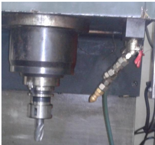
(c) Step 2: Milling of each layer to required layer
