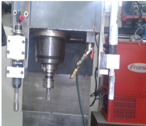
(a) Pneumatic hammer, milling cutter and welding torch assembly on 3-axis CNC machine
