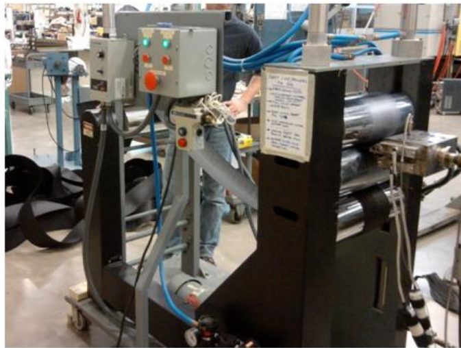
Figure 2: Extrudate being fed into the 3-Roll Mill
